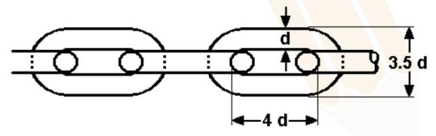
Chain lengths from 3D to 9D are currently in use. Shorter link chains require more links, and are heavier and more expensive, more so, it exists the possibility that a shorter link would not accept a determined size of shackle. On the other hand, shorter links are easier to handle with a winch and are a little more wear resistant. Longer chain links are less propense to knotting and easier to handle with a hook.
