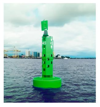
The manufacturing process of the elastomer buoy float is based on a solid rolled body of closed-cell polyethylene foam sheet and bound by heat. No chemical substance is involved in it.
