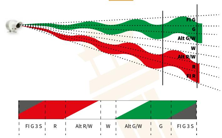
As can be observed on the image, the main advantage of this type of sector light, is that the information about the deviation in reference to the center of the channel is progressive and quantitative. Considering that a bigger deviation will alter the flashing proportion between colors. That is, in the green/white sector, a bigger deviation will result in a bigger proportion of green light, and a smaller deviation will increase the duration of white flashes.
