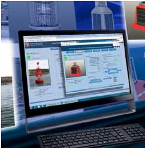
GLOBAL NETCOM is a Remote Monitoring Multicentre that provides an easy way to obtain information and interacts with the different remote stations installed in lighthouses, buoys and beacons, displaying the data in a clear way on a computer screen.
