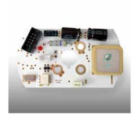
MFGPS position and synchronisation module is a device with double function. On the one hand, it is used to determine buoy positioning and, on the other hand, to synchronise lanterns through a GPS receiver of 12 channels.
